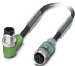
Sensor/actuator cable, 3-position, Variable cable type, Plug angled M12, A-coded, on Socket straight M12, A-coded, with 2 LEDs, cable length: Free input (0.2 ... 40.0 m)
