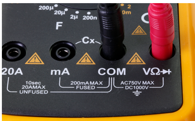
Figure 1-20 Sockets on one more meter.
