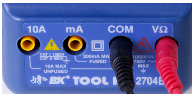
Figure 1-18 Note the labeling of sockets on this meter.
