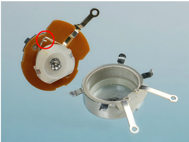
Figure 1-50 The wiper of the potentiometer is circled.
