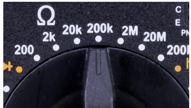
Figure 1-23 A manual meter requires you to select the range.
