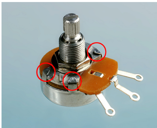
Figure 1-48 The tabs that hold a potentiometer together.
