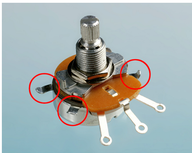
Figure 1-49 The tabs have been bent upward and outward.
