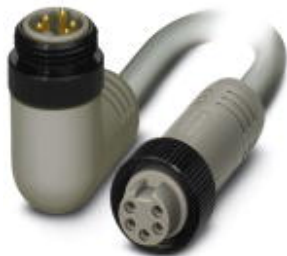
Bus system cable, DeviceNet™, 5-position, PVC, gray, Plug angled 7/8"-16UNF, A - standard, on Socket straight 7/8"-16UNF, A - standard, cable length: 20 m
