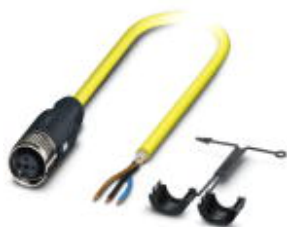
Sensor/Actuator cable, 3-position, PVC, yellow, shielded, free cable end, on Socket straight M12 SPEEDCON, A-coded, Cable length: 10 m
