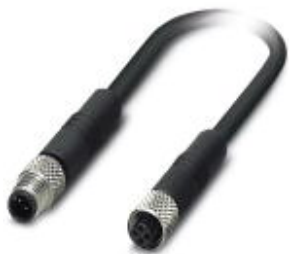
Sensor/Actuator cable, 3-position, PUR, black RAL 9005, Plug straight M5, A-coded, on Socket straight M5, A-coded, Cable length: 0.2 m
