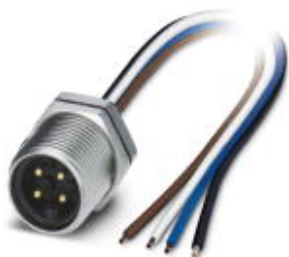
Sensor/actuator flush-type plug, 4-pos., 7/8", rear mounting with 7/8" fastening thread, with 1.0 m PE litz wire, 4 x 0.75 mm 2
