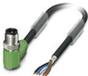
Sensor/actuator cable, 5-position, Variable cable type, shielded, Plug angled M12, A-coded, on free cable end, cable length: Free input (0.2 ... 40.0 m)
