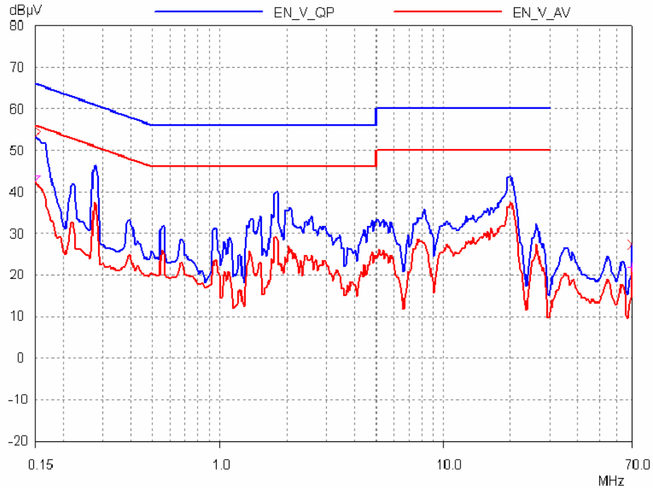
Figure 33 – Conducted EMI, Maximum Steady State Load, 90 VAC, 60 Hz, and EN55022 B Limits.
