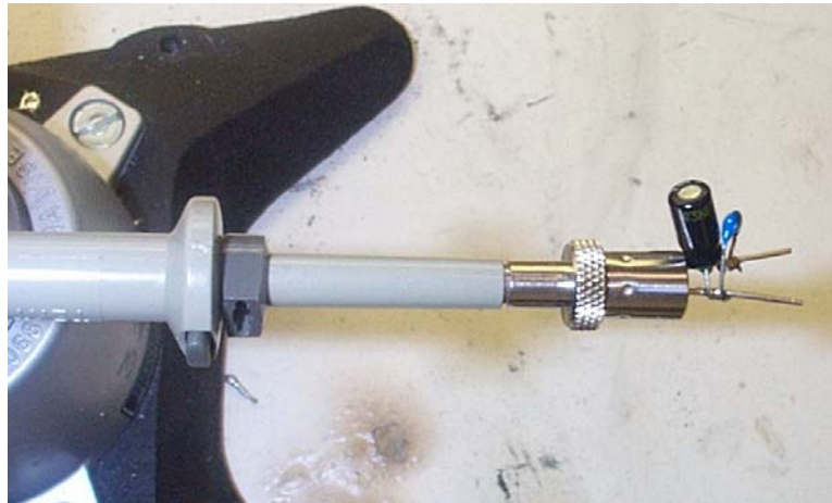
Figure 28 – Oscilloscope Probe with Probe Master ( www.probemaster.com ) 4987A BNC Adapter. (Modified with wires for ripple measurement and two parallel decoupling capacitors added)
