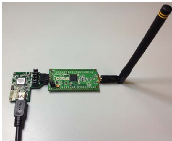
Figure 1 ADuCRF101 Mini Board and Emulator Board
