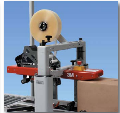
Tapes dispense and seal cases easily by hand, hand-held dispenser, or with a semi-automatic or fully automatic case sealer.
