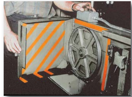
Orange 3M™ Vinyl Tape identifies dangerous machine parts when enclosure doors are open. 131
