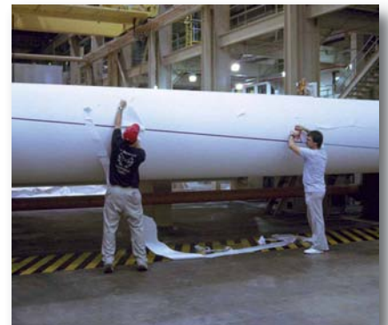
For finished mill overlap splicing, 3M™ Repulpable Permanent Tape 900B provides high shear strength without adhesive oozing or bleed through.
