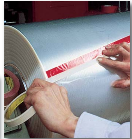
With high tack and good shear strength, 3M™ Double Coated Tape 9420 splices plastic film quickly and securely. Red carrier identifies the splice for later removal.
