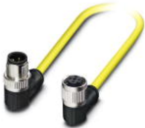
Sensor/Actuator cable, 4-position, TPE, yellow RAL 1021, Plug angled M12 SPEEDCON, A-coded, on Socket angled M12 SPEEDCON, A-coded, Cable length: 5 m
