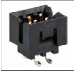
Vertical SMT, dual row shrouded header with centre locking window and dual side slot
