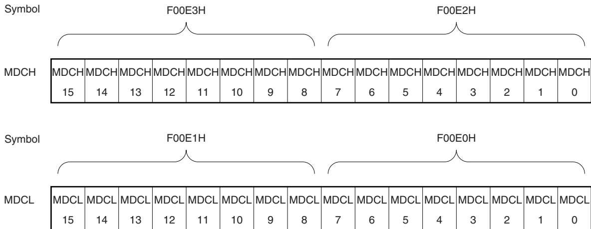
Figure 13-4. Format of Multiplication/Division Data Register C (MDCH, MDCL)
