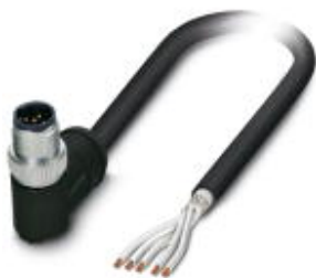
Sensor/Actuator cable, 5-position, PE-X halogen-free, black, shielded, Plug angled M12 SPEEDCON, A-coded, on free cable end, Cable length: 10 m, For railway applications
