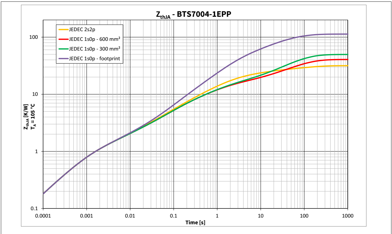
Figure 9 Typical Thermal Impedance. PCB setup according Chapter 4.4.1
