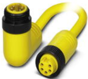
Power cable, 5-position, PVC, yellow, Plug angled 7/8"-16UNF, on Socket straight 7/8"-16UNF, cable length: 5 m
