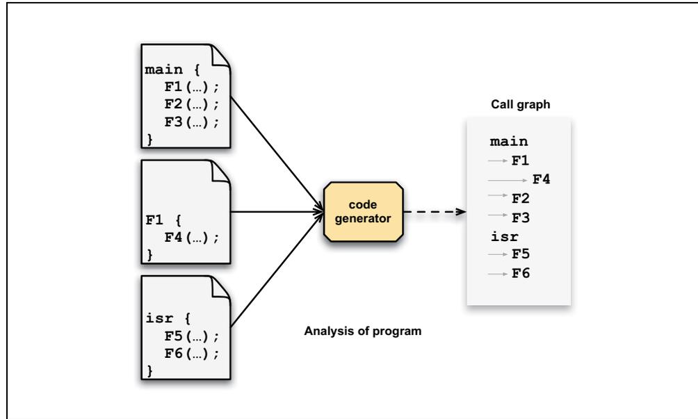
Figure 5-1 shows sections of a program being analyzed by the code generator to form a call graph. In the original source code, the function `main()` calls `F1()`, `F2()` and `F3()`. `F1()` calls `F4()`, but the other two functions make no calls. The call graph for `main()` indicates these calls. The symbols `F1`, `F2` and `F3` are all indented one level under `main`. `F4` is indented one level under `F1`.
