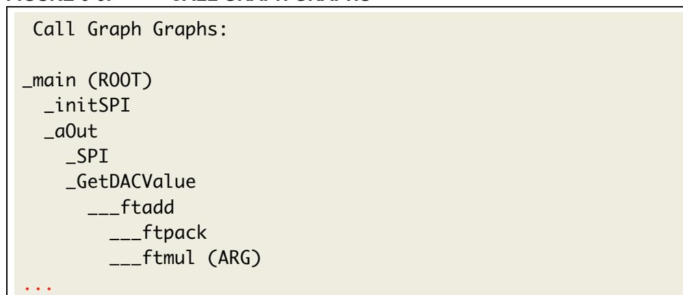
Indentation is used to indicate the call depth. In the diagram, you can see that `main()` calls `aOut()`, which in turn calls `GetDACValue()`, which in turn calls the library function `__ftadd()`, etc. If a star (\*) appears next to the function's name, this implies that the function has been called indirectly via a pointer.
