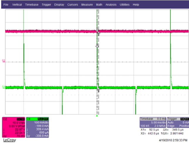
Figure 36 – 230 VAC, 6° Phase. Upper: V_{OUT} , 10 V / div. Lower: I_{IN} , 0.1 A / div., 5 ms / div.
