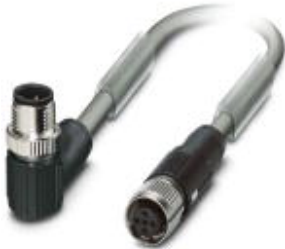
Bus system cable, CANopen®, 5-position, PUR halogen-free, Gray RAL 7001, shielded, Plug angled M12-SPEEDCON, A-coded, on Socket straight M12-SPEEDCON, A-coded, Cable length: 1 m
