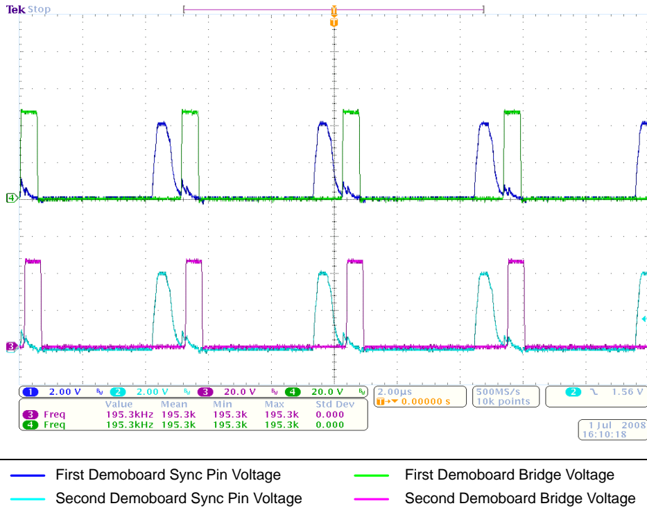
Figure 21. Synchronized – Sync Pins Connected
