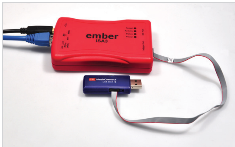
Figure 2: USB Stick and ISA3 Connection
