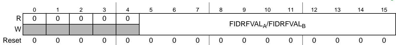
Figure 21-62. Receive FIFO Frame ID Rejection Filter Value Register (RFFIDRFVR)
