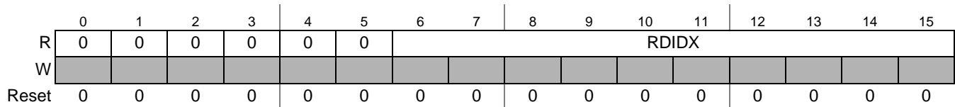
Figure 21-58. Receive FIFO B Read Index Register (RFBRIR)
