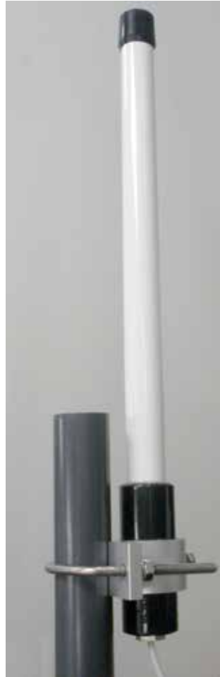
Figure 41. Mast Mount Antenna – Side View with Attachment to Pipe
