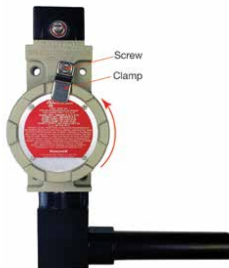
Figure 47. Switch Battery Replacement
