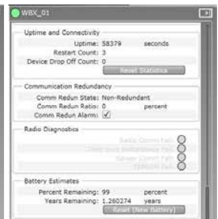
Figure 31. Battery Estimates on Property Panel
