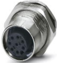
Sensor/actuator flush-type socket, 8-pos., M12 SPEEDCON, rear/screw mounting with Pg9 thread, with straight solder connection
