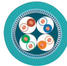
Ethernet, flexible, CAT5e [94B]
