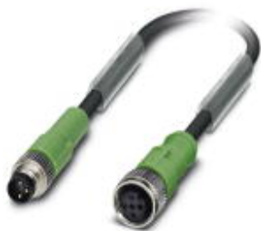
Sensor/actuator cable, 3-position, Variable cable type, Plug straight M8, on Socket straight M12, A-coded, cable length: Free input (0.2 ... 40.0 m)
