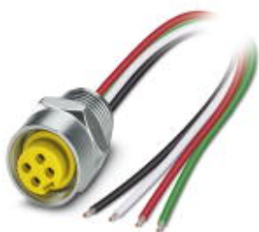
Flush-type connector, 4-position, Socket, straight, 7/8"-16UNF, on free cable end, Front mounting, with 1/2 inch-14 NPT mounting thread, Individual wires, cable length: 1 m
