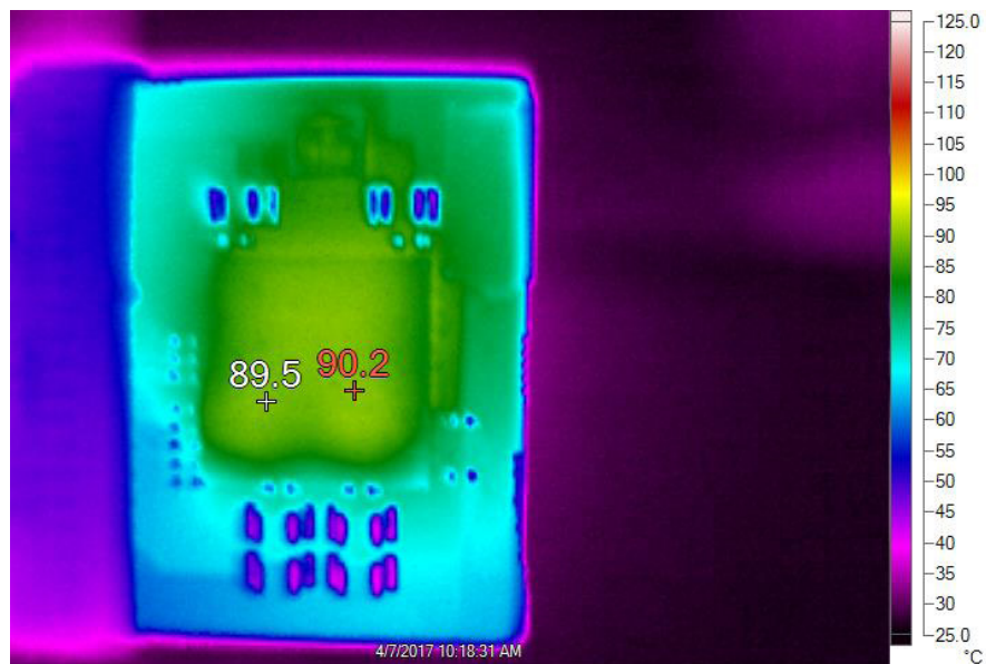
Figure 7. Thermal Performance at V_{IN} = 12V , V_{OUT1} = 3.3V/15A , V_{OUT2} = 2.5V/15A , f_{SW} = 600kHz , T_A = 23^\circ C , 400LFM Airflow
