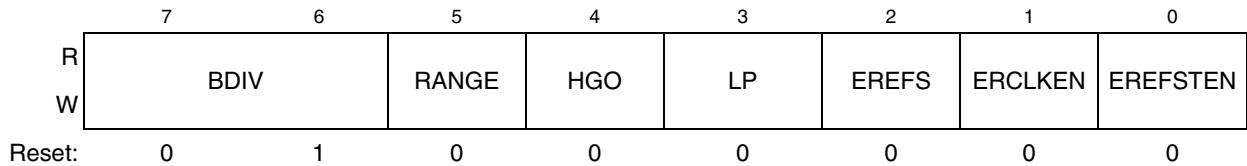
Figure 19-3. ICS Control Register 2 (ICSC2)
