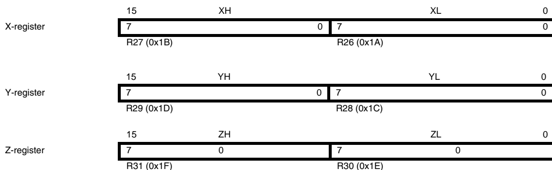
Figure 5-5. The X-, Y-, and Z-registers
